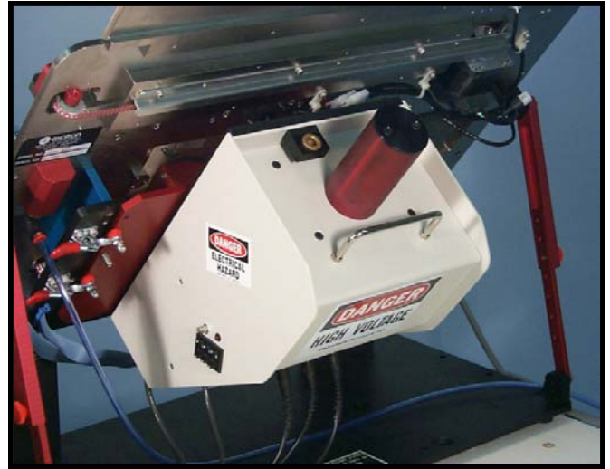
Backside of handler Test head docked into place
