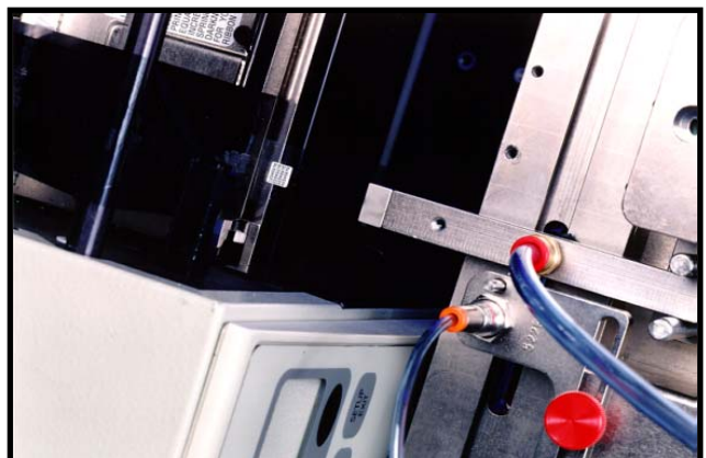
Pick & Place label applicator Eliminates ESD problems with direct peel label application methods
