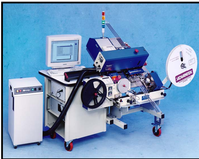
JDS Uniphase YAG Laser Marker
