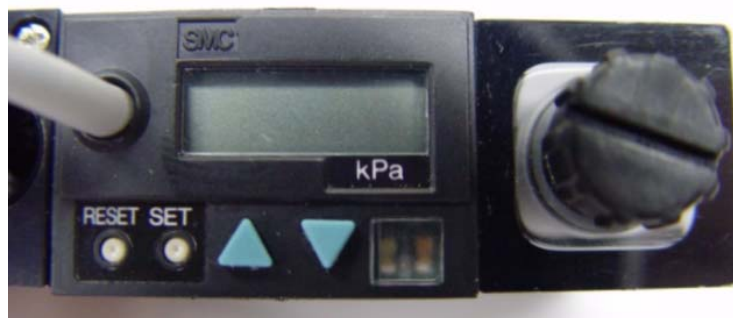
Figure 6-1: Vacuum Generator Closeup
