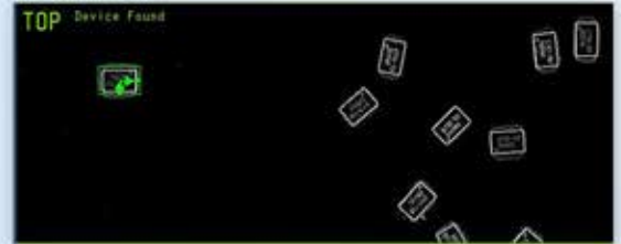
Top inspection locates and identifies devices
