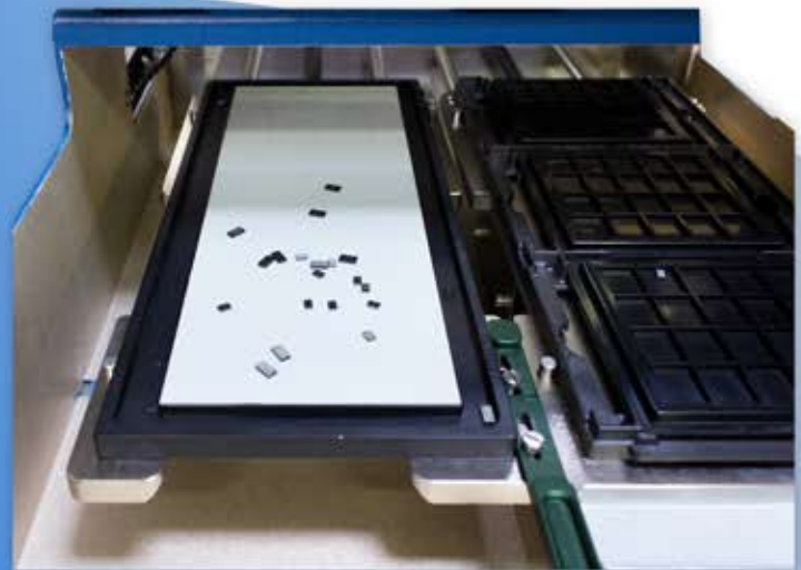
Devices are presented scattered on the input tray and sorted by device size to the output tray or tape
