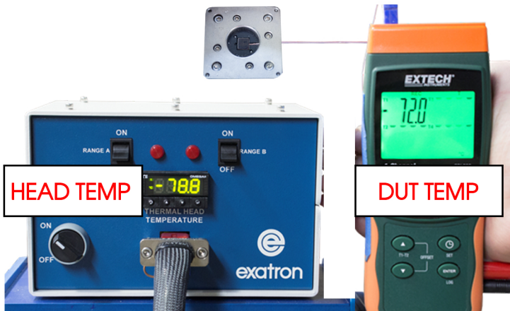
Actual Test Temperatures - QFN with Embedded Thermocouple
