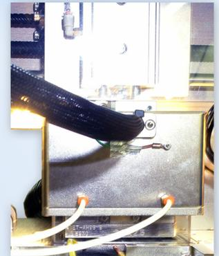
Double-sided Cold Test with Purge Enclosure
