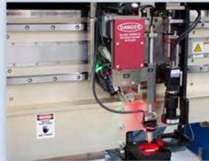
Linear Motor-Driven XYZ Pickup Head
