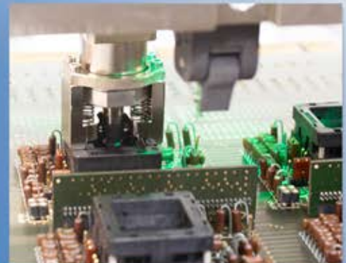
Pusher Pickup Head Opens/Closes Open Top Sockets
