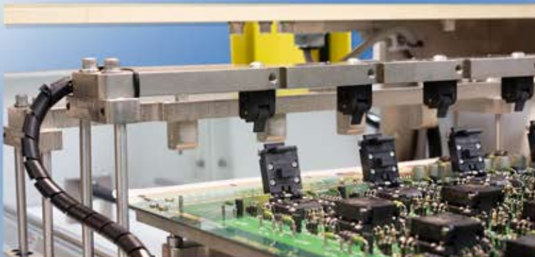
Lifter Fingers (front) and Pusher Blocks (back) Open/close Clam Shell Sockets
