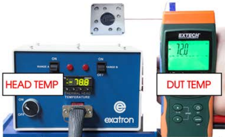
Actual Test Temperatures - QFN with Embedded Thermocouple
