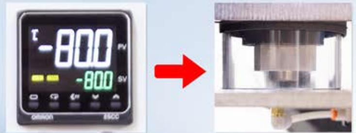
Even at -80°C there is no frost on the test head.
