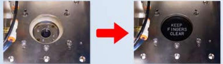
Shutter is open only during device removal/replacement
